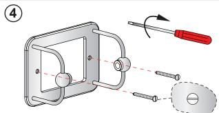
Screw in the stainless steel screws to secure the base to the wall.
