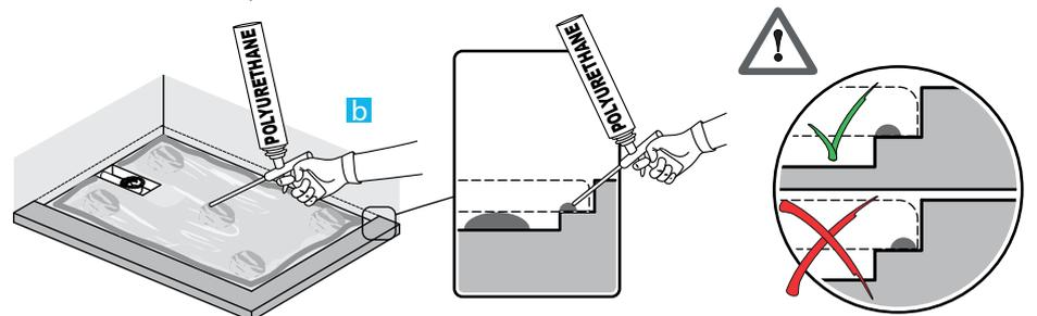
MONTAGGIO CON PIEDINI - ASSEMBLY WITH FEET - MONTAGE AVEC PIEDS - MONTAGE MIT FÜSSEN - MONTAJE CON PATAS - MONTAGE MET Pootjes - ΤΟΠΟΘΕΤΗΣΗ ΜΕ ΠΟΔΑΡΑΚΙΑ - МОНТАЖ НА НОЖКАХ - MONTÁŽ S NOŽKAMI - MONTÁŽ S NOŽIČKAMI - MONTAŽA Z NOGAMI - MONTAŽA S NOŽICAMA
