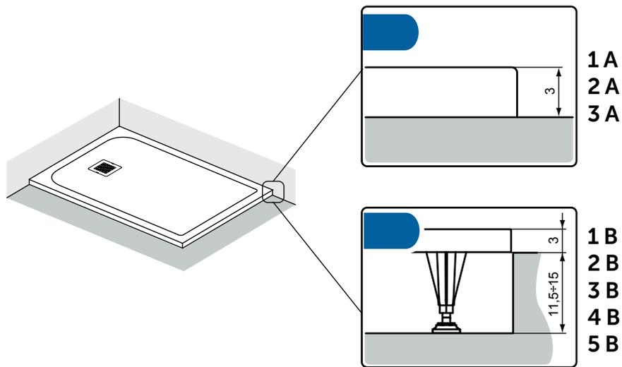
**MONTAGGIO AD INCASSO - BUILT-IN ASSEMBLY - MONTAGE À ENCASTREMENT - EINBAU - MONTAJE EMPOTRADO -
