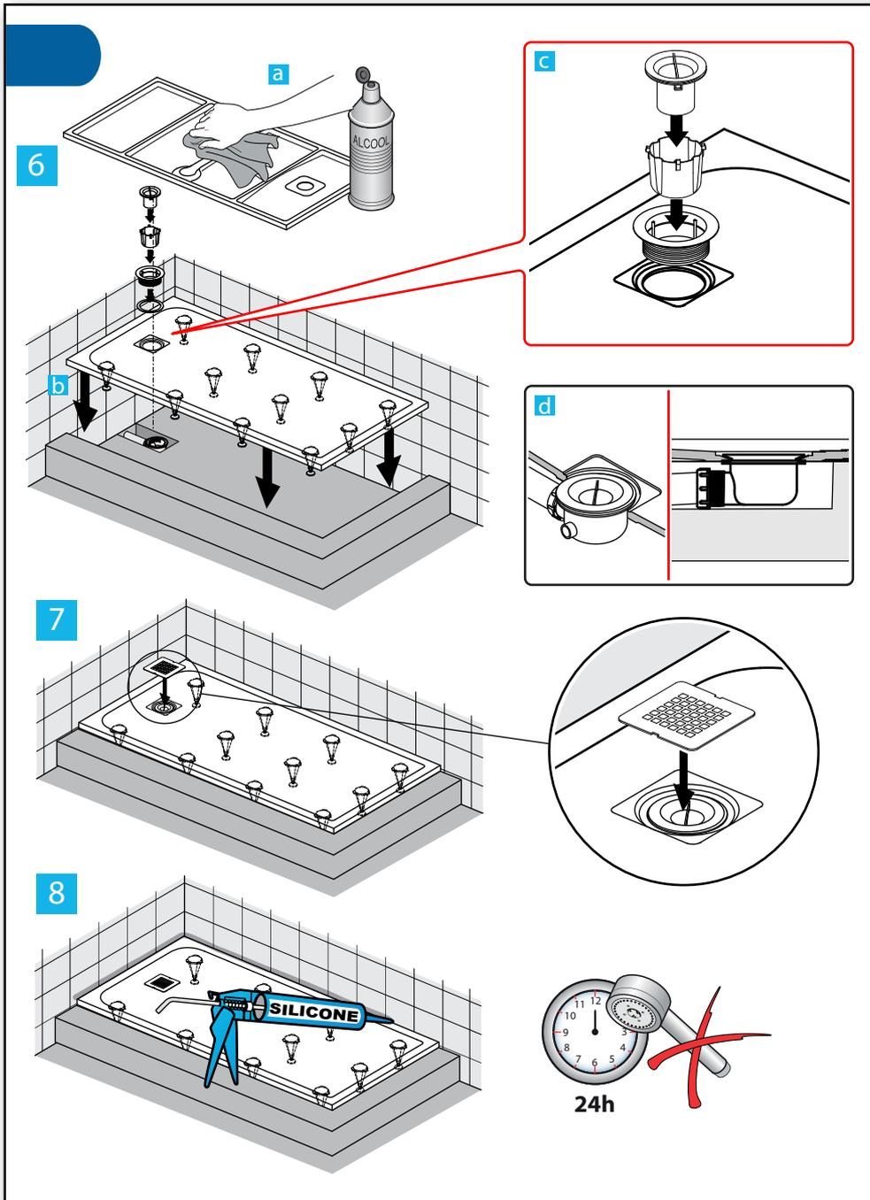
MONTAGGIO A INCASSO - BUILT-IN ASSEMBLY -
