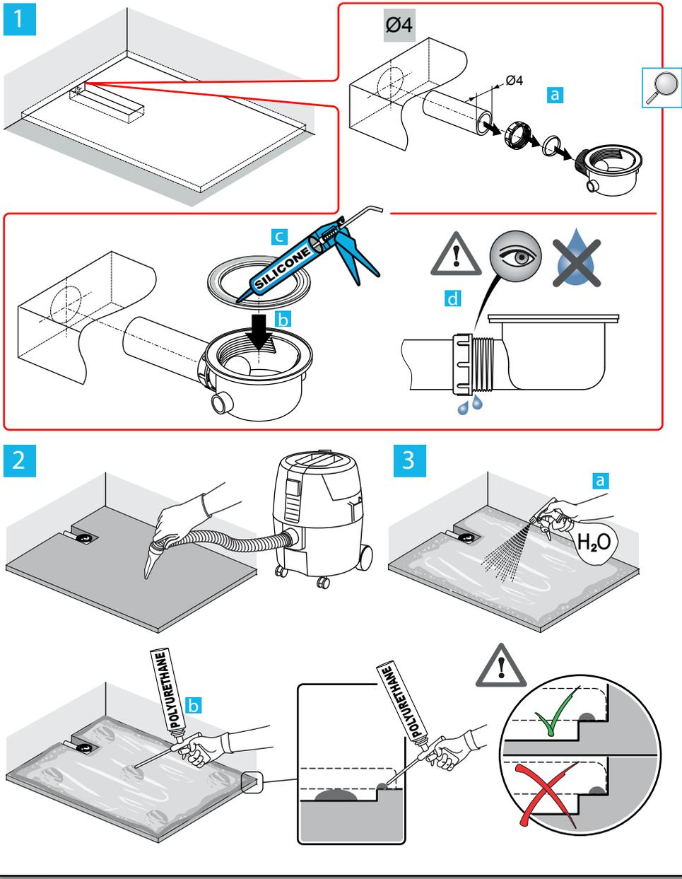
MONTAGGIO A PAVIMENTO CON PIEDINI - FLOOR ASSEMBLY WITH FEET - MONTAGE AU SOL AVEC PIEDS - MONTAGE MIT FÜSSEN - MONTAJE CON PATAS - MONTAGE MET Pootjes - ΤΟΠΟΘΕΤΗΣΗ ΜΕ ΠΟΔΑΡΑΚΙΑ - МОНТАЖ НА НОЖКАХ - MONTÁŽ S NOŽKAMI - MONTÁŽ S NOŽIČKAMI - MONTAŽA Z NOGAMI - MONTAŽA S NOŽICAMA
