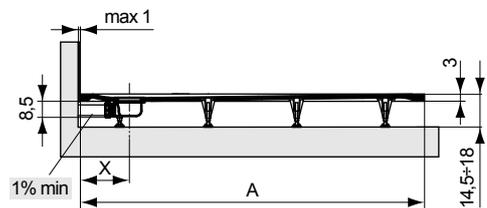
MONTAGGIO A INCASSO - BUILT-IN ASSEMBLY - MONTAGE À ENCASTREMENT - EINBAU - MONTAJE EMPOTRADO -
